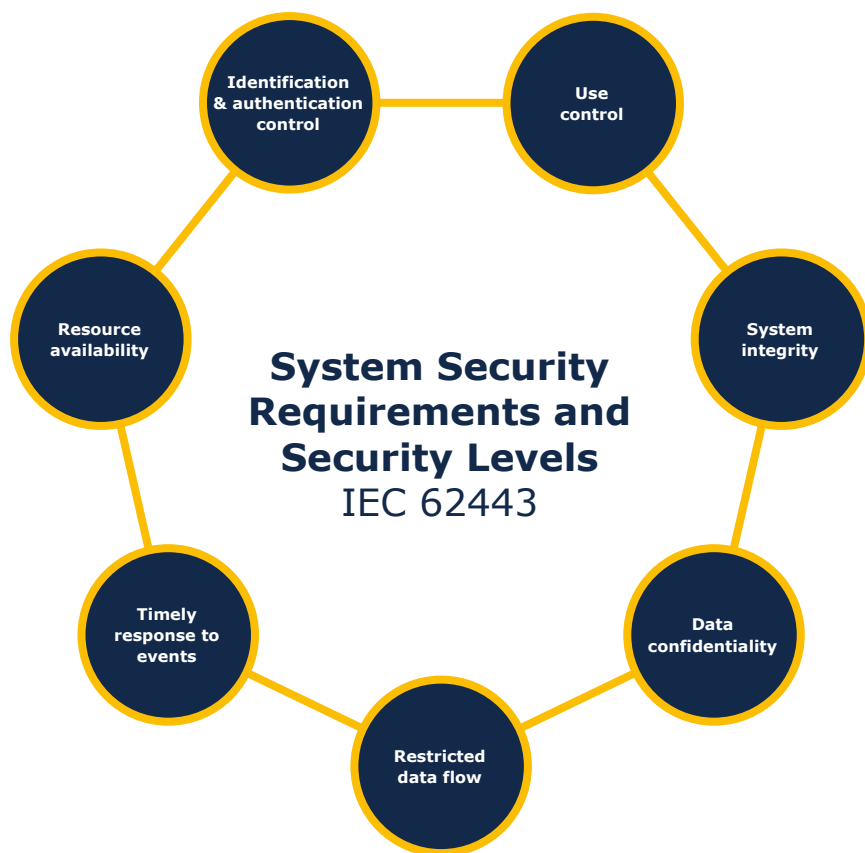
Exhibit 4.1: System security requirements and security levels according to IEC 62443 [Source: Axon Consulting, based on IEC 62443]
